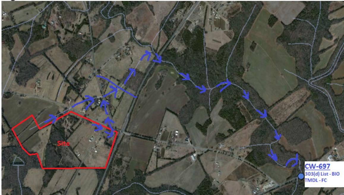
Figure 2.2: Stormwater Runoff Route
