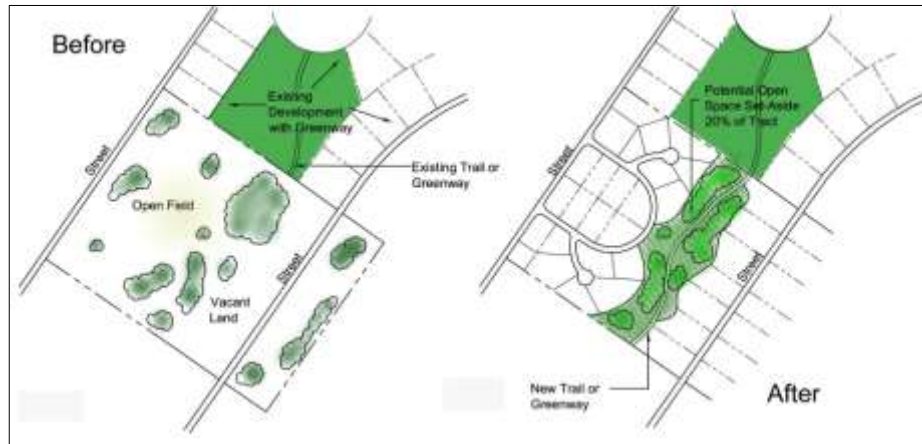
Figure 26-5.4(e): Example Open Space Set-Aside Configuration
