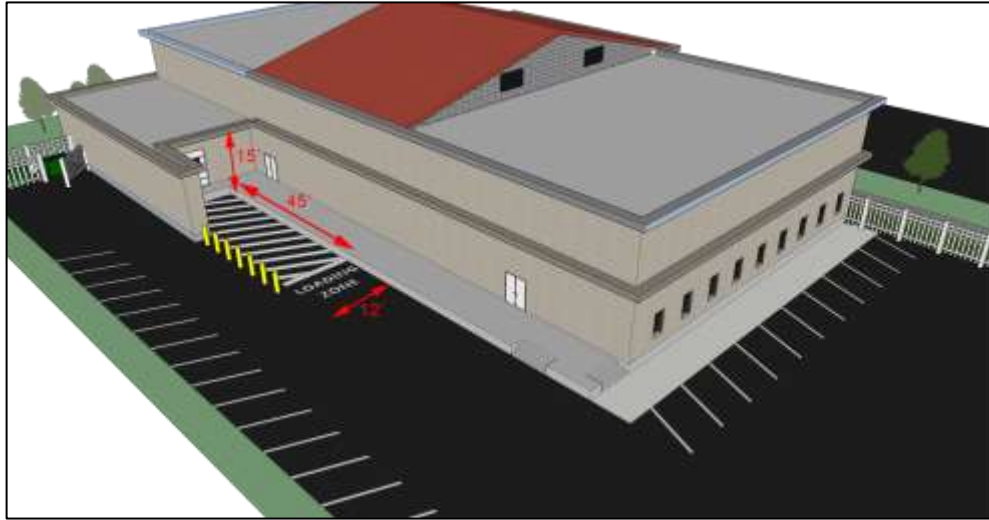
Figure 26-5.2(j): Loading Area Configuration
